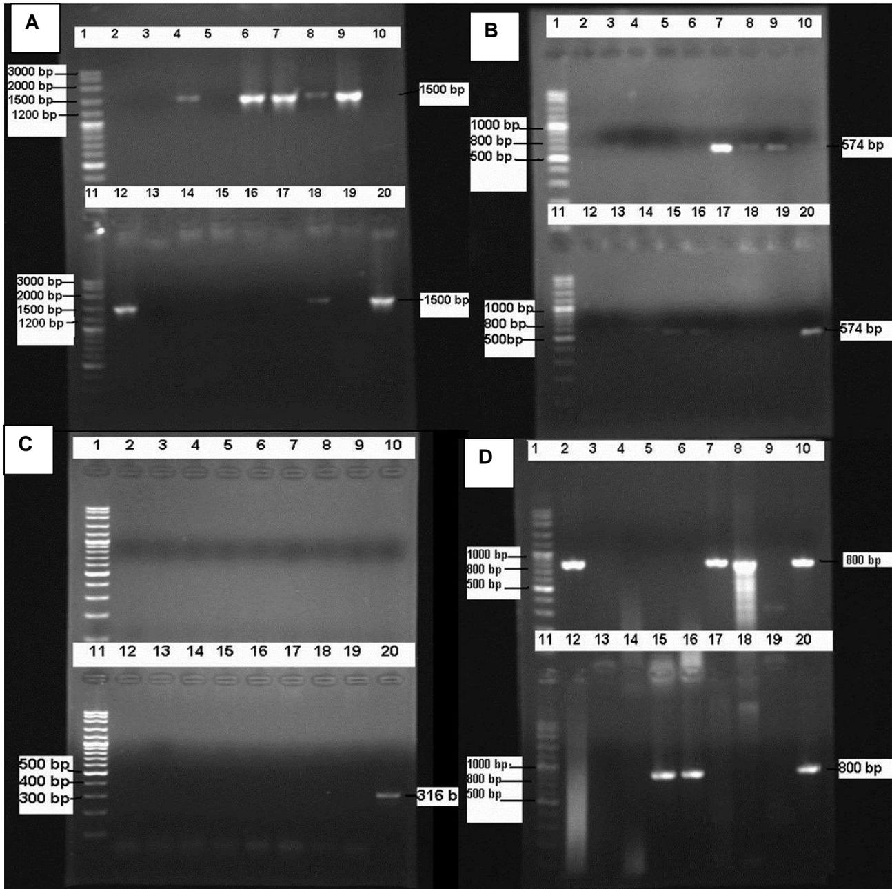
Fig. 1. Molecular detection (PCR and RFLP) of *Mycoplasma* species from sheep in Khanozai, district Pishin, Balochistan. A, *M. mycooides* cluster showing an amplicon size of 1500 bp; B, members of *M. mycooides* sub cluster showing an amplicon size of 574bp; C, *Mycoplasma capricolum* subsp *capripneumoniae*. showing an amplicon size of 316bp; D, *Mycoplasma putrifaciens* (*Mp*) showing an amplicon size of 800bp.
