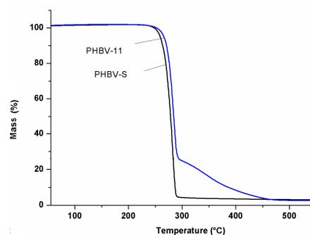
Fig. 8. TG thermogram of PHBV-S and PHBV-11.
