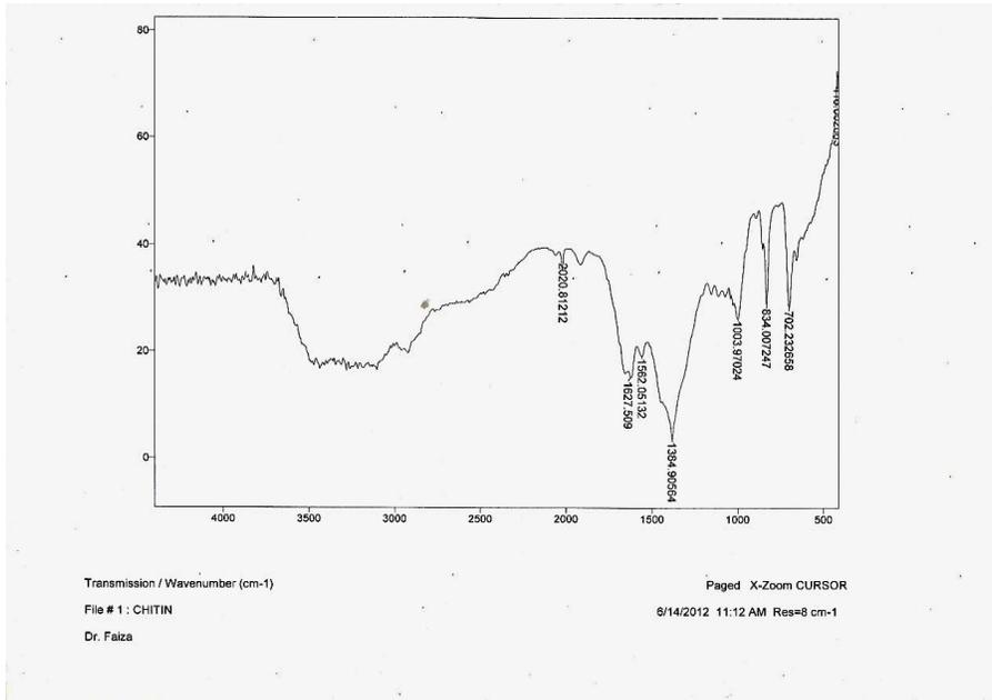
**Fig 1: FTIR analysis of chitin purified from shrimp shells.**
